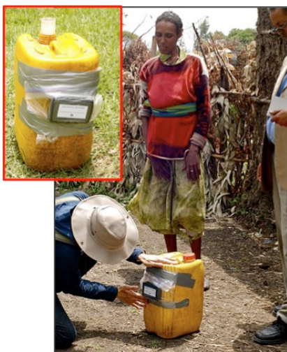
Figure 8: Researcher attaching the WuhaGize sensor, encased in a black box, to a water container. The inset shows the sensor attached to the water container.
