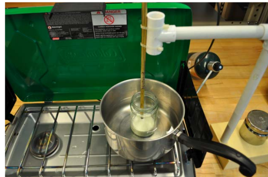
Figure 5: Flash heat pasteurization setup in the lab.
